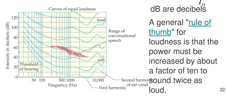
A decibel is one tenth of a **bel** (**B**). Devised by engineers of the Bell Telephone Laboratory to quantify the reduction in audio level over a 1 mile (1.6 km) length of standard telephone cable, the bel was originally called the *transmission unit* or *TU*, but was renamed in 1923 or 1924 in honor of the laboratory's founder and telecommunications pioneer Alexander Graham Bell. In many situations, however, the bel proved inconveniently large, so the decibel has become more common.
