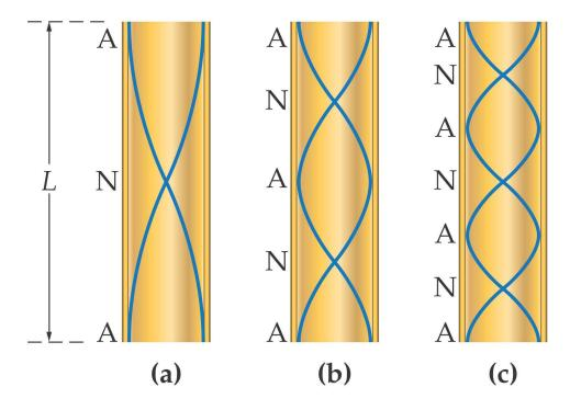
The next standing wave pattern to satisfy the conditions at the ends of the pipe will have one more node and one more antinode than the previous standing wave. Its wavelength will be L.
