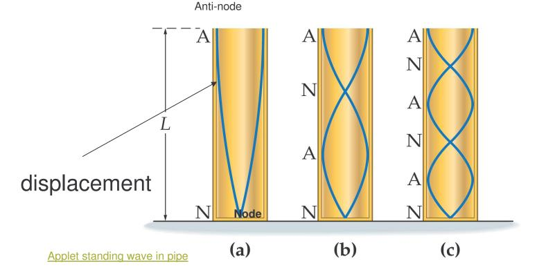
One end of the pipe is a pressure node, the other a pressure antinode. The distance between a consecutive node and antinode is one-quarter of a wavelength.
