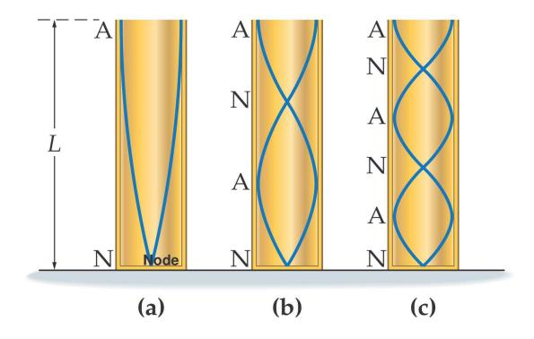
The next standing wave to satisfy the conditions at the ends of the pipe will have one more node and one more antinode than the previous standing wave. Its wavelength will be (4/3)L.
